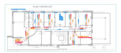
Vacuum Lines for Suction Machines, use only 45° elbows, laying with 1% Slope.
